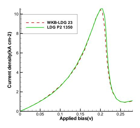
Figure 6: Comparison between the reference solution and the WKB-LDG solution: the I-V characteristics of a RTD. 23 cells are used in the WKB-LDG method.
