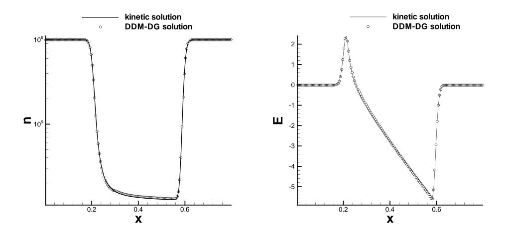
Figure 3: The global kinetic simulation (solid line) versus the DDM-DG solution (circles). Left: the concentration n; right: the electric field E.
