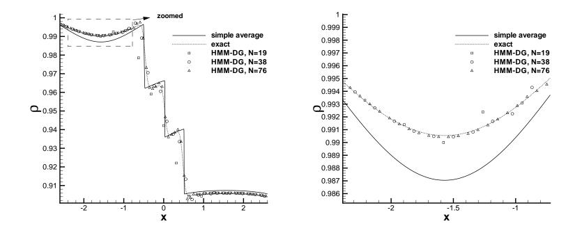
Figure 2: Sod's Shock tube problem. Density  $\rho$ . The HMM-DG solution with N=19, 38 and 76 uniform elements for  $\varepsilon=10^{-6}$ , versus the converged "exact" locally averaged solution  $\bar{u}$  to the nonlinear oscillatory Euler equations. The solution  $\tilde{u}$  of the simply averaged Euler equations (simple average) is also plotted as a reference. Left: the solutions in the whole interval; right: zoomed around x=-1.5.
