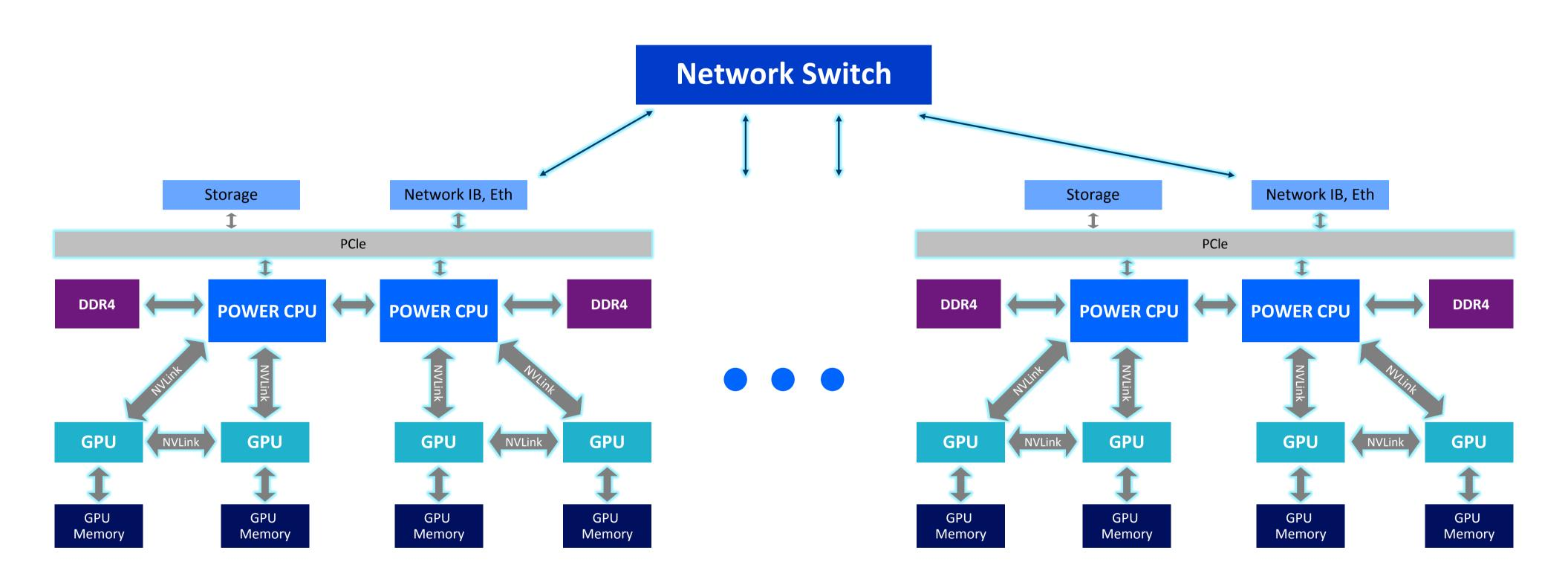
Power Al DDL: Fully utilize bandwidth for links within each node and across all nodes
